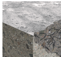
Steel fiber concrete
