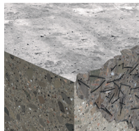
Steel fiber concrete
